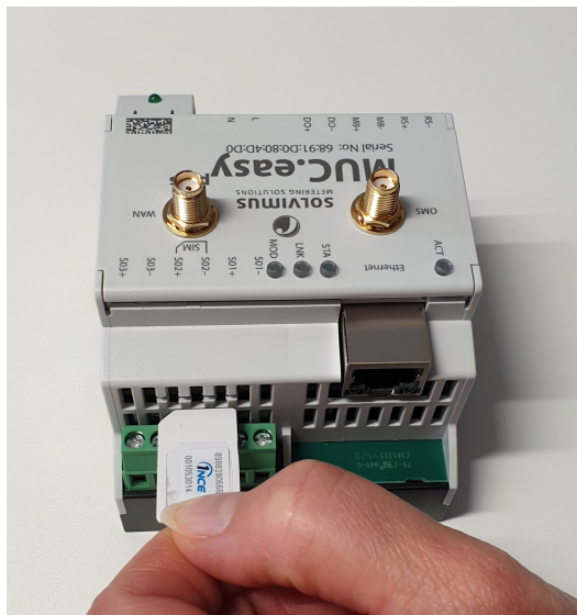
Figure 3: Insertion of the SIM card in a device with integrated mobile network modem
