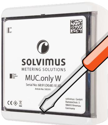
Insert a flathead screwdriver (blade width approx. 3 mm) into the recess of the latch on the bottom.
