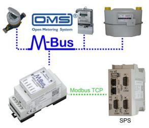
The devices of the MBUS-GEM product family come with a standard Ethernet interface which supports Modbus TCP in slave mode. The controlling system as a Modbus master is therefore able to access the data of the meters directly using Modbus registers via the connected network. This can also be done in remote or distributed applications.
