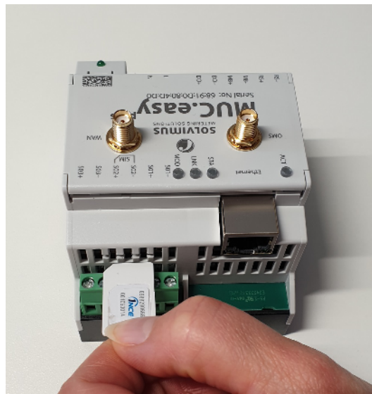
Figure 2: Insertion of the SIM card in a device with integrated mobile network modem
