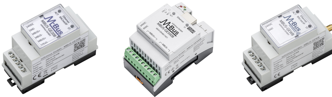
Figure 1: MBUS-GEB in the wired and wireless variants
