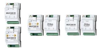
As most installations are composed of both wired and wireless meters, the wireless MUC500 W has, in addition to the radio receiver, an additional interface for connecting an external level converter for the wired M-Bus. When combined with a level converter MBUS-PS500, both M-Bus and wM-Bus can be read out.
