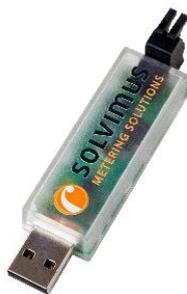
One product that is especially developed for temporary reading and the field service is our level converter MBUS-PU3. It converts from USB to M-Bus. This enables mobile devices like Smartphones or laptops to communicate directly with the meter. The device is entirely bus-powered by the USB port.
