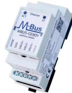
Our MBUS-GE20V and MBUS-GE80V are two level converters for remote applications. They can handle up to 20 or 80 unit loads and are translating the serial data into data packets sent via Ethernet. The IP network allows having the remote device on-site or far-off. A simple TCP socket (or optional a virtual COM port; we recommend the driver from company Eltima) on the data terminal end is used for transparent M-Bus communication over Ethernet.
