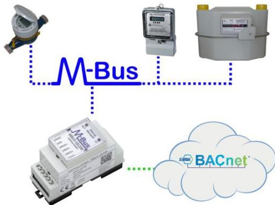
The gateways of the MBUS-GEB product family come with a BACnet software stack which is certified according to PICS (BACnet/IP Annex J). This ensures the compatibility with other BACnet devices.
