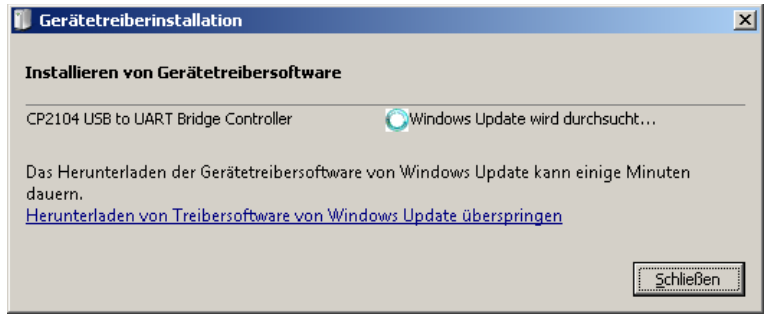
Figure 4: Driver installation upon first connect of the MBUS-PU3 to the host system
