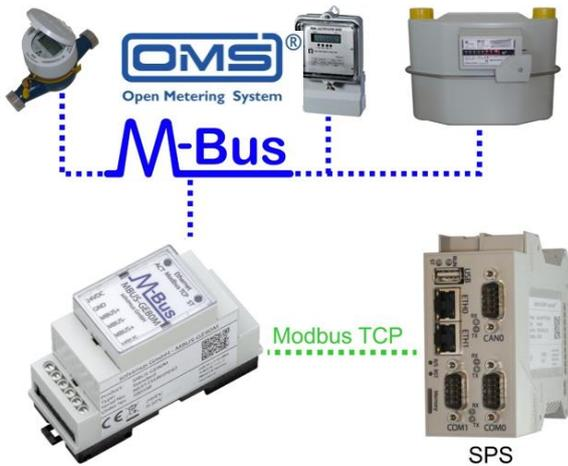
The devices of the MBUS-GEM product family come with a standard Ethernet interface which supports Modbus TCP in slave mode. The controlling system as a Modbus master is therefore able to access the data of the meters directly using Modbus registers via the connected network. This can also be done in remote or distributed applications.
